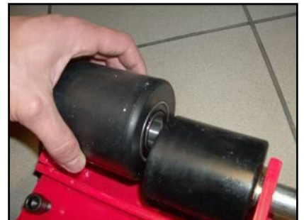
Figure12 – Removing the wheel.
