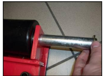
Figure10 – Seeger retainer for wheel pins.
